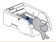
When the countdown finishes (factory setting: 1 minute), the cleaning rake will be activated.
